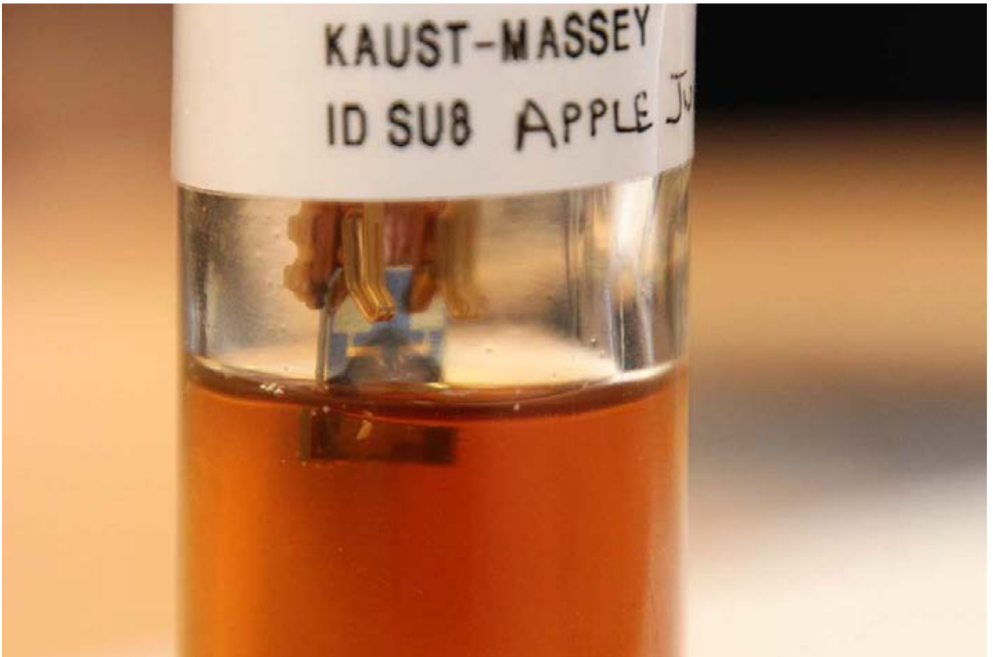
The DEHP sensor immersed in a sample of apple juice.
