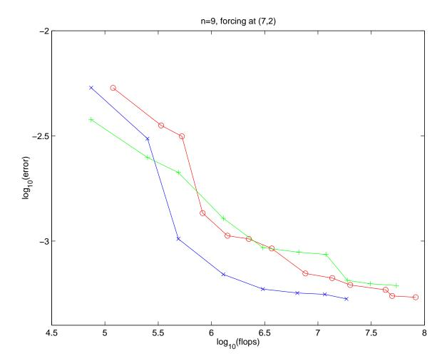
Figure 8: Log-log plot of the error as a function of the number of floating point operations needed to integrate the reduced system of equations for a time of 0.1s. "+" is the flat Galerkin, "o" is for integration on the AIM, while "x" refers to the post-processed case.
