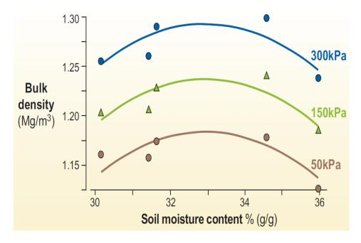
*Figure 2.* Proctor test compaction curves for the Timaru silt loam at three contrasting applied pressures.
