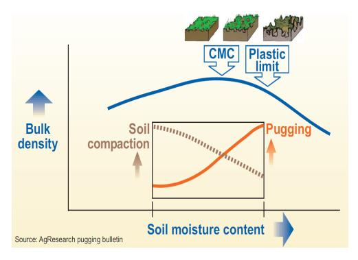
Figure 1. The relationship between achievable bulk density and soil moisture
