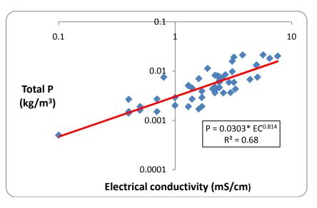
Figure 6: Electrical conductivity and phosphorus concentrations (log transformed).
