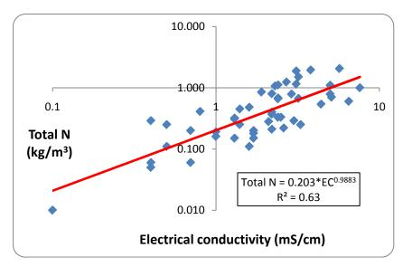
Figure 5: Electrical conductivity and nitrogen concentrations (log transformed).
