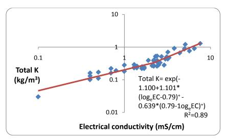
Figure 7: Electrical conductivity and potassium concentrations (log transformed).
