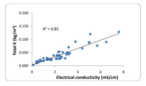
Figure 4: Electrical conductivity and potassium concentrations.
