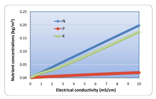
**Figure 8:** Calculated nutrient concentrations for given electrical conductivity reading. Note that nutrient concentration estimates above EC 7.6 mS/cm have been extrapolated.
