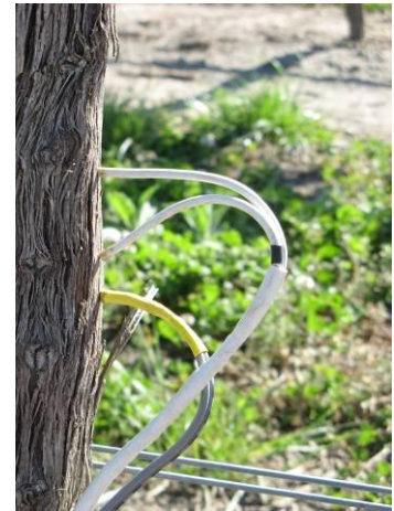
Figure 2. Sap flow sensors have been used to measure the actual water use ( ET_C , symbols) of the grapevines in Marlborough. The basal crop factor ( K_C , vines only) was calculated from the ratio of ET_C to ET_0 . The value of K_C is about ( \sim 0.45 ) for these grapevines because of the sparse leaf canopy.
