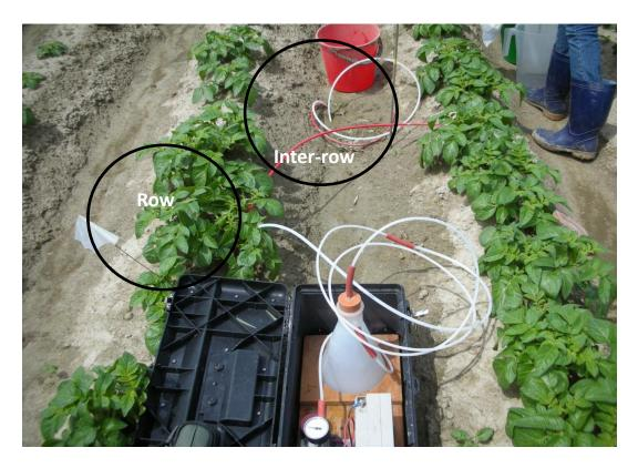
Figure 2 Extraction of drainage by connecting the tube to a pump. Each fluxmeter has two tubes to the surface, the white one to collect the water and the red for air entry and escape.
