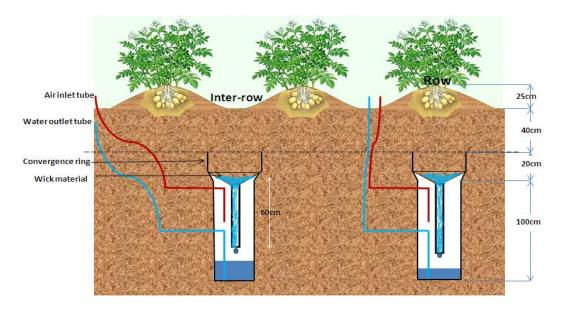
Figure 1. A schematic diagram showing fluxmeters installed under the row (right) and interrow (left) in the potato field
