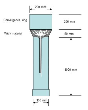
Figure 1. Passive wick lysimeter to monitor water and nutrient fluxes.
