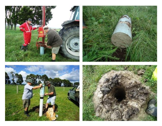
Figure 2. Preparation and installation of drainage flux meters
