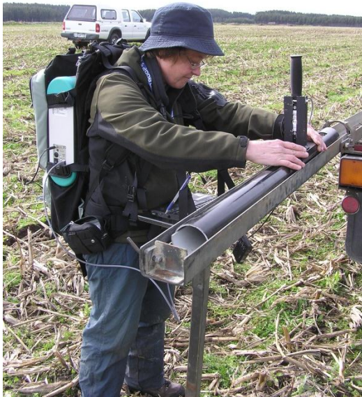
Figure 3. Scanning a core in the field, with some examples of the produced spectra.
