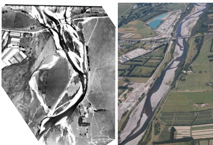
Figure 2. The lower Otaki River has been straightened and narrowed by river engineering approaches since the 1950s implemented for flood protection. It provides a typical example of the reduction in geomorphic and habitat complexity in many previously laterally active gravelly rivers in NZ: (a) 1939, (b) 2013 (SH1 bridge for reference in the top of each photo).
