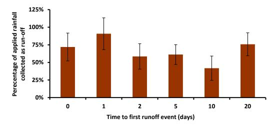
**Figure 1.** Percentage of applied rainfall collected as runoff. Figures have been averaged across all soil monoliths receiving water on a given day. Error bars represent 1 Std Dev.
