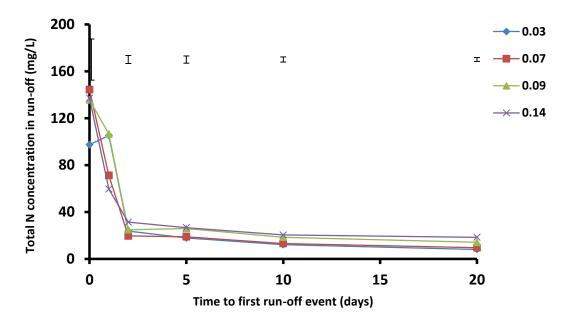
**Figure 3.** Total nitrogen (N) concentration (mg/L) in runoff following the application of manure of varying dry matter content and time till first runoff event. Error bars represent LSD<sub>(5%)</sub>. Statistical differences between concentrations on Day were not determined due to large variation between replicates.
