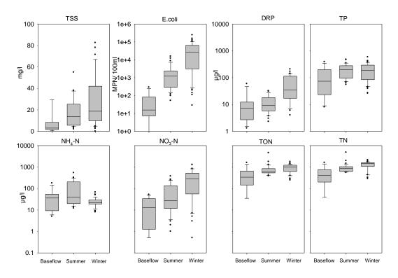
Figure 4 Box plots of TSS, E. coli and different forms of P and N at the lower wetland weir.
