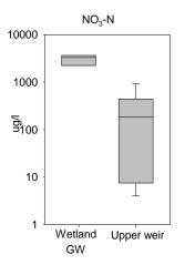
**Figure 5** Box plots of NO<sub>3</sub>-N during baseflow for the wetland subsurface flow immediately upstream of the upper weir and for the upper weir.
