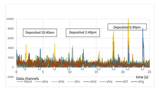
**Figure 2.** Detection of urine patches placed at various times during the day and detected at 7pm that day, dry soil, damp surface. Blue marks below zero indicate the placement of a urine patch.
