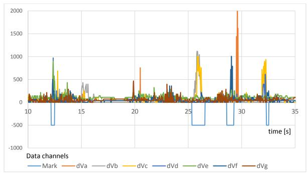
Figure 6. Urine patch detection in dry soil, data collected 2 hours after placement.
