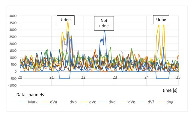
**Figure 4.** Comparison of response to urine and dung patches, dry soil, damp surface. The signal amplitude is increased with moist soil, as can be seen in Fig. 5, where the data was collected in late spring before this summer's drought had started.
