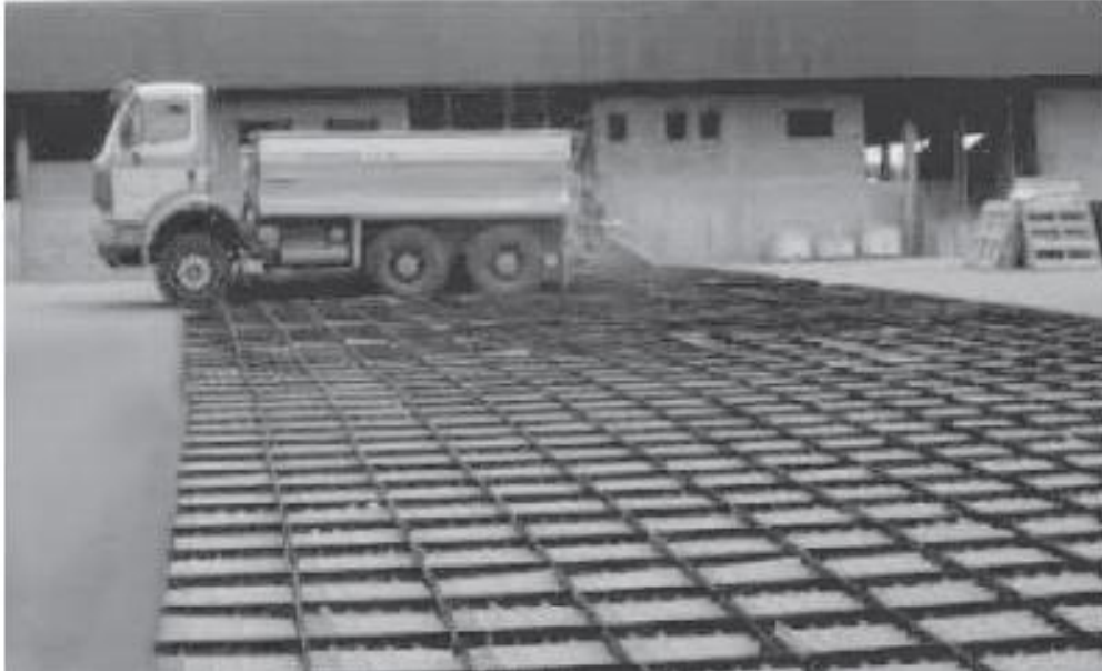
Figure 1: 1400 tray matrix used to collect 18 simultaneous transverse tests on a Transpread “W” twin chain spreader (Lawrence 2006)
