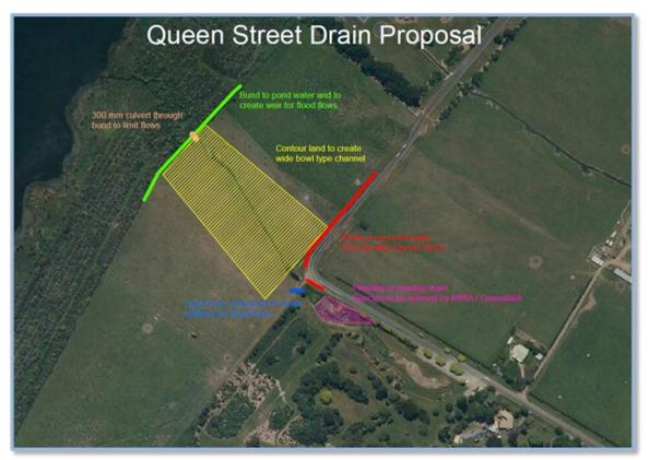
Figure 3: Draft design proposal to filter stormwater from the Queen street drain before it enters Lake Horowhenua.
