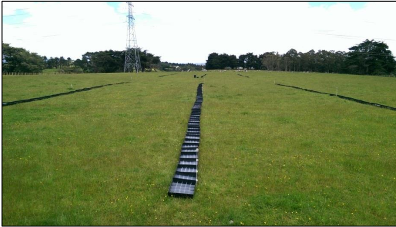
Figure 1: Distribution of trays in a flat paddock prior running the Spreadmark tests.
