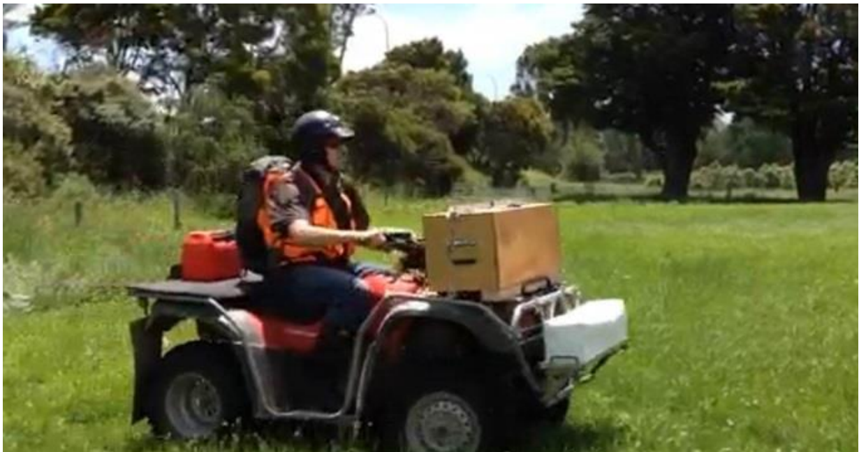
Fig. 3 Mobile gamma soil survey system
