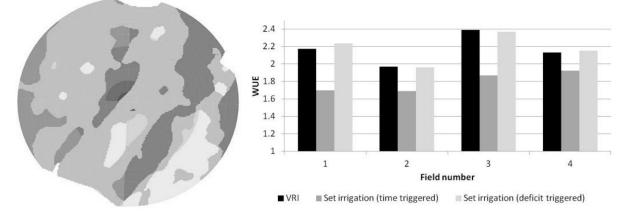
*Figure 2* Example outputs of water use efficiency (WUE) in wheat under a centre pivot irrigator with multiple irrigation strategies (VRI, triggered by elapsed time, triggered by soil water deficit), considering spatial variability in soil properties and cropping management in a ficticous test scenario.
