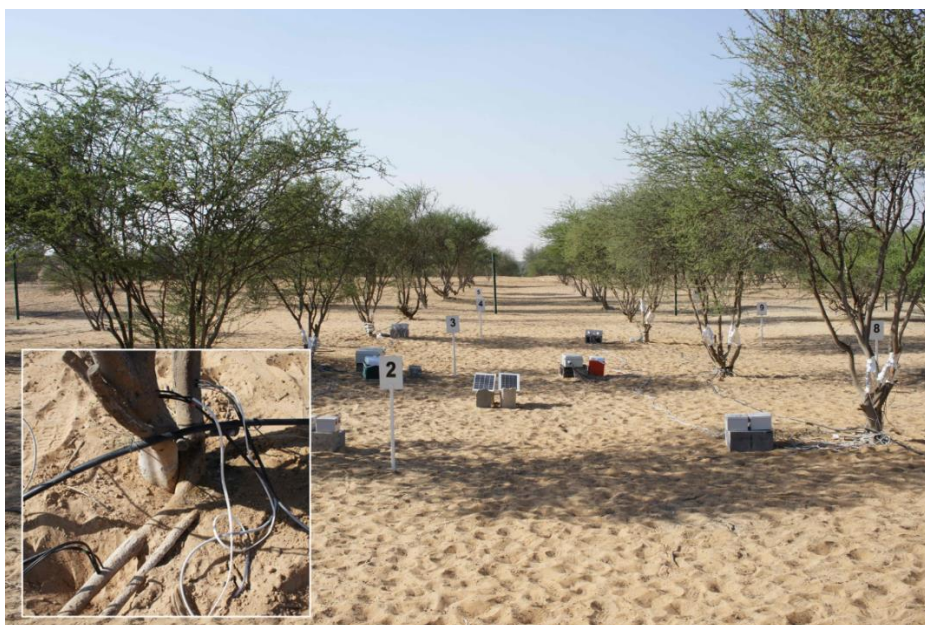
Figure 7. The experimental plot of Samar ( Vachellia tortilis ) trees near Madinat Zayed, Abu Dhabi. The inset shows a set of heat-pulse probes in a transverse surface root.
