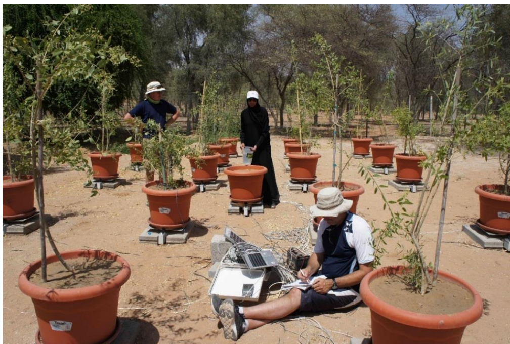
Figure 5. The experimental plot of Arak ( Salvadora persica ) trees growing in weighing lysimeters, near Al Ain in Abu Dhabi.
