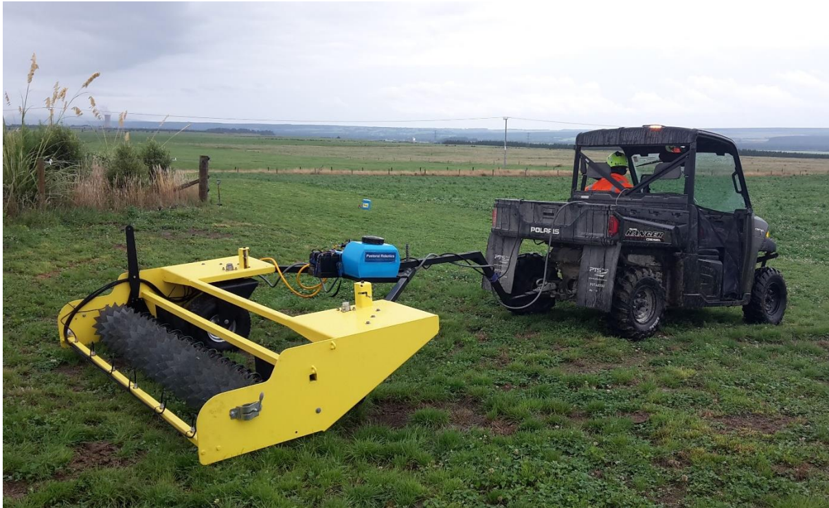
Fig. 6. A 2.8m-wide Spikey® trialling on a Landcorp farm, towed by a side-by-side.
