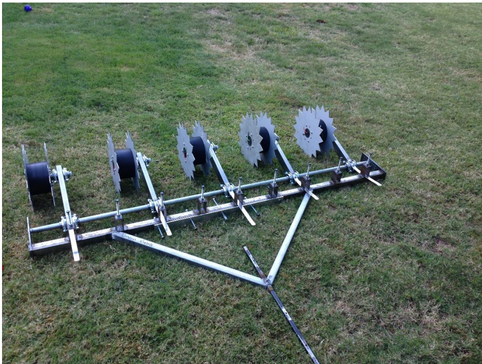
Fig. 1. An early small hand-pulled device for detecting urine patches.
