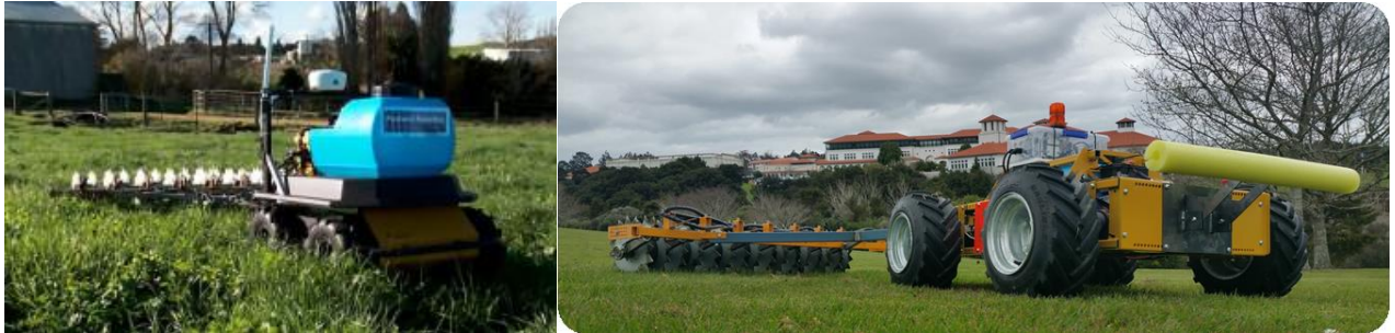
Figs 9a and 9b. Original imported and Massey University-built prototypes of the Mini-ME® autonomous robotic tow vehicle.
