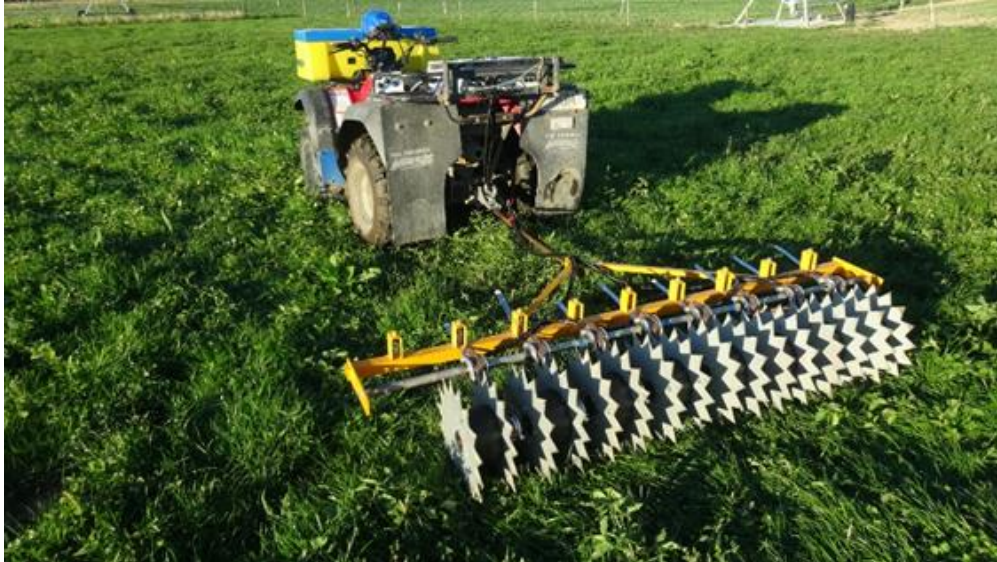
Fig. 2. The 1.8m-wide ‘Spikey’ device being towed by quad-bike.
