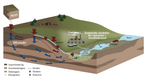
Figure 2: Concept figure of the Danish national nitrogen model (from Højberg et al., 2015)
