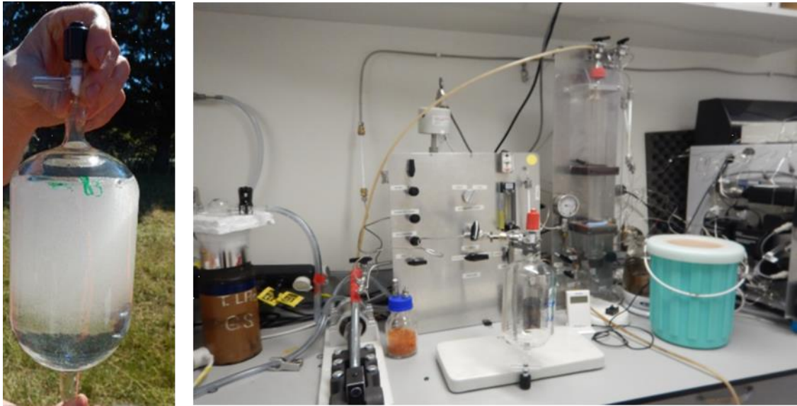
Figure 3: (a) Full Ne flask during sampling (left). (b) syringe and chromatography inlet system (right).
