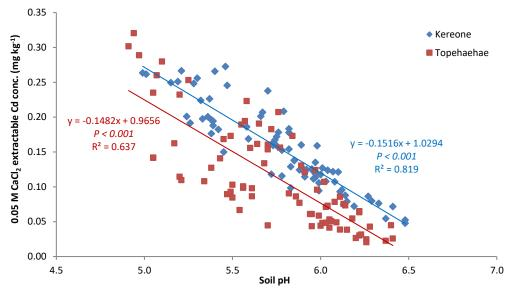
**Figure 2**. Relationship between soil extractable Cd concentration and soil pH for the Kereone and Topehaehae soil types.
