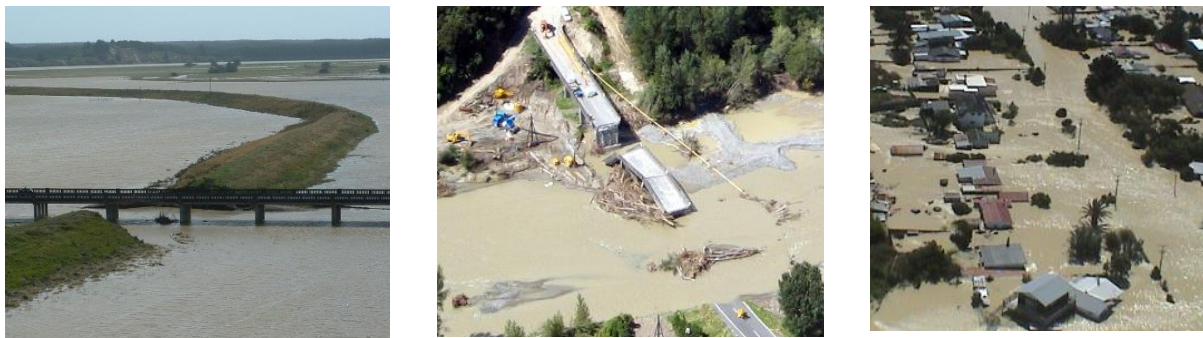
Downstream damage caused by the storm included breached stopbanks, broken bridges and hundreds of flooded houses.
