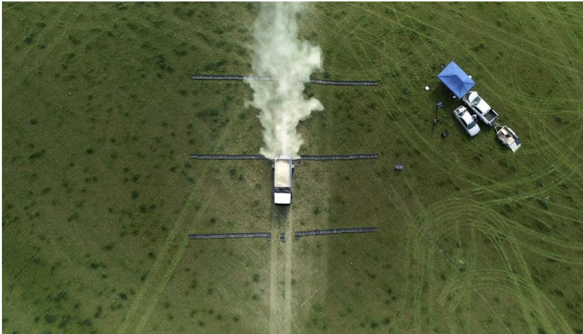
Figure 2: Overhead view of truck L during a trial, showing layout of 3 collection lines. Photo provided by Victoria O’Sullivan of Ravensdown.
