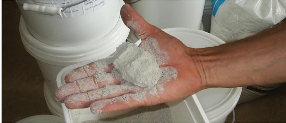
Figure 1: Example of squeeze test with a moist sample of lime, from Lincoln Agritech testing in 2004.
