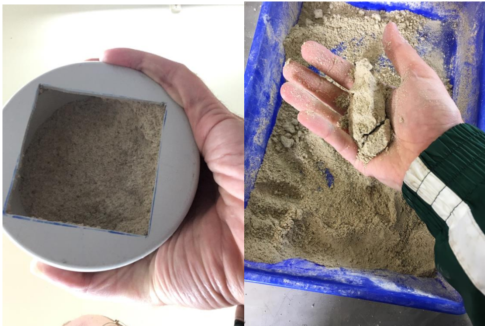
Figure 4: The packed lime sample is then inverted to check its flowability. If it does not easily flow out (as shown at left) it is considered unsafe to load. This has found to correlate well with clumping of lime in the pilot’s squeeze test (right).
