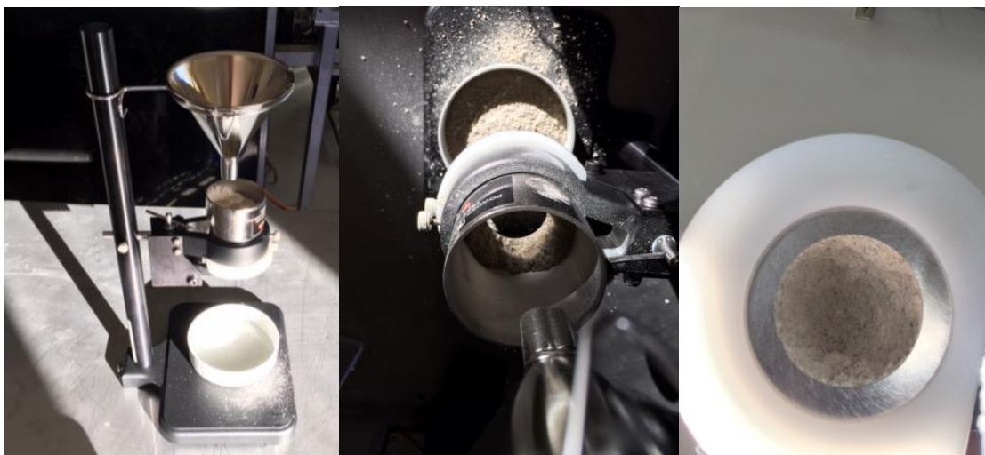
Figure 2: Left – Flodex device; Center – lime sample passing orifice; Right – lime lodged inside (bottom view)
