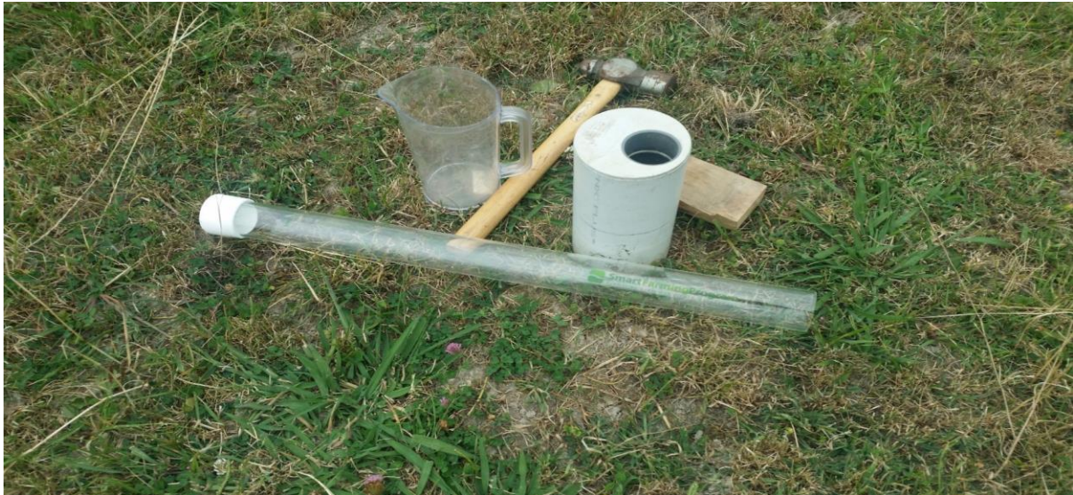
Figure 3 Smartfarms environmental monitoring kit including water clarity tube and soil water infiltration measurement device
