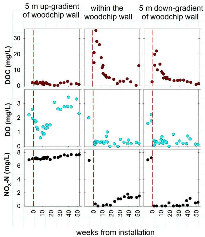
**Figure 1:** Time-series for water chemistry parameters: dissolved organic carbon (DOC), dissolved oxygen (DO) and nitrate, measured in groundwater up-gradient; within, and down-gradient of the woodchip wall. Hatched line marks the time of woodchip wall installation.
