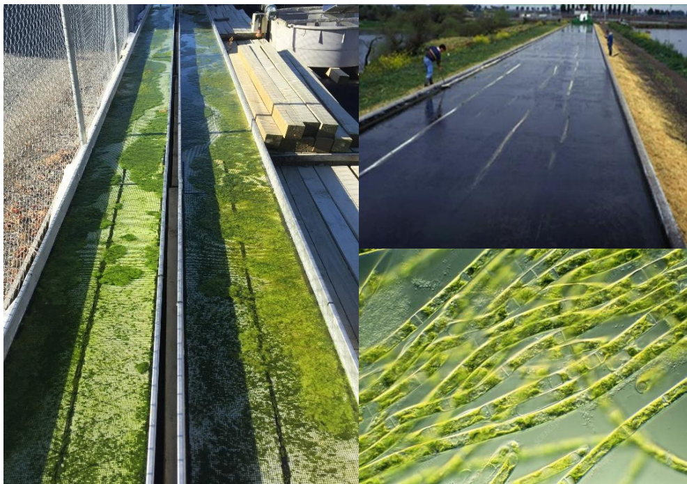
Figure 20: Filamentous Algal nutrient scrubbers being trialled at pilot scale in Waikato (left) and field scale in California, USA (top right). Close-up of filamentous algal (bottom right). (Photos: Rupert Craggs)
