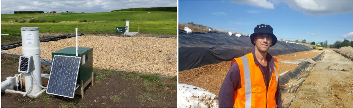
Figure 24: Woodchip bioreactors treating tile drainage at Waituna, Southland (left; photo C. Tanner) and stream flow at Barkers Creek, South Canterbury (right; photo RadioNZ 2019).
