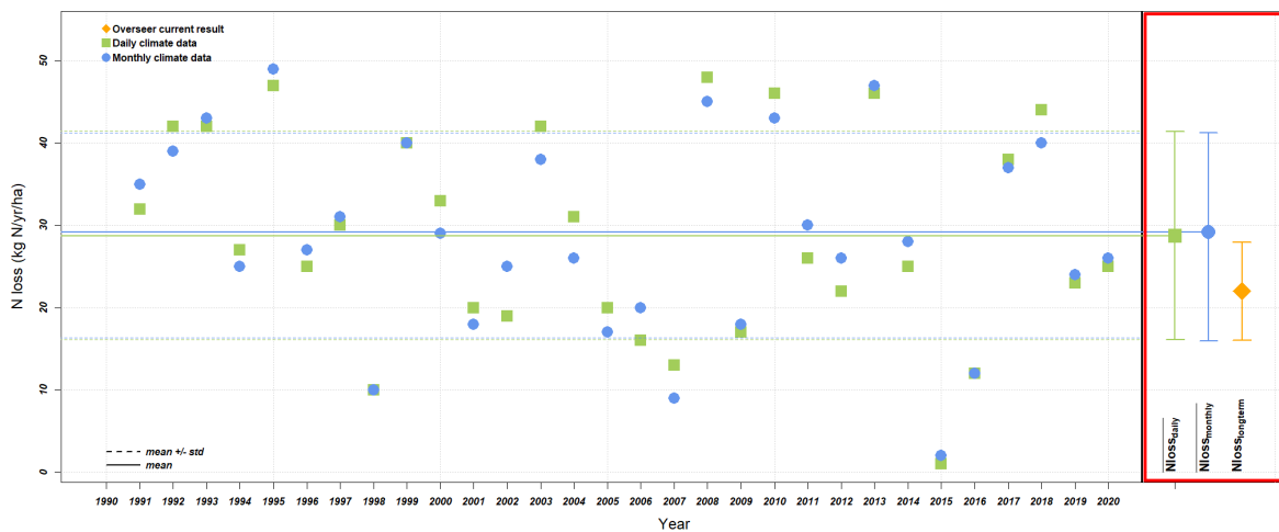
Figure 2: 30 years of annual N-loss estimates from DVal (blue) and MVal (green). Means (solid lines) and standard deviations (dotted lines) are represented by the coloured lines and projected into error bars in the red rectangle. The long-term N-loss estimate with uncertainty (Overseer, 2022a) is indicated in orange.
