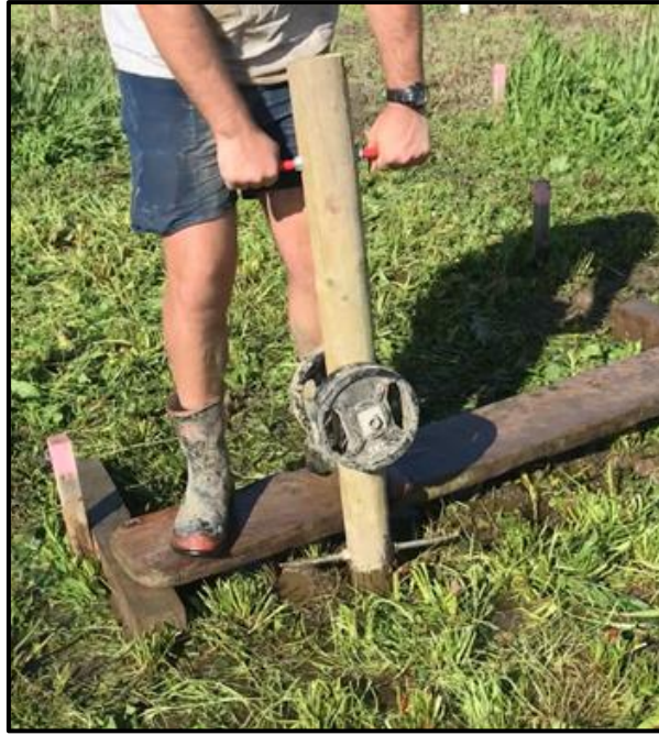
Photo 5: The puggo-stick, with 20kg of weights attached to it.
