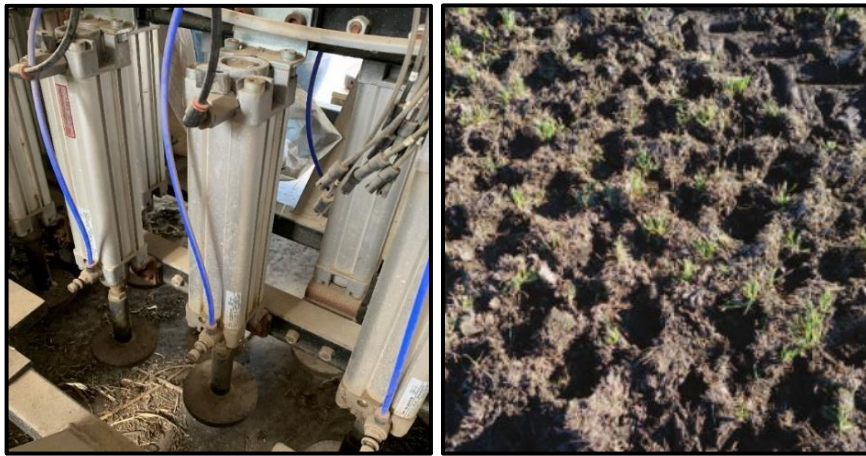
Photo 4: Left: The hydraulic rams and treading plates of the hoofinator (Photo: Richard Gillespie, New Zealand Institute for Plant and Food Research, Lincoln). Right: Treading damage to un-tilled pasture plots by the hoofinator at 261kpa (Hu et al. 2018).
